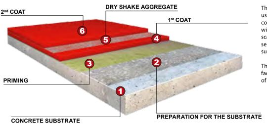
These systems are normally made using combinations of floor coatings or flow-applied flooring with intermediate aggregate scatter, colour and nature selected over a fresh coating surface.
